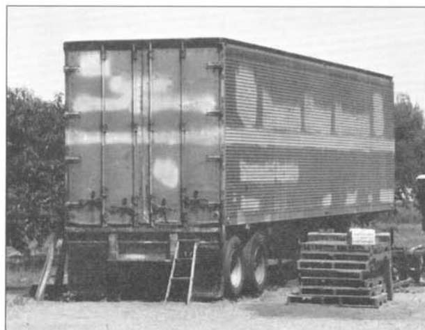
Figure 2. Refrigerated highway van used as a cold room.
